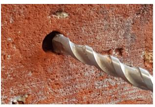
To countersink the screw head, drill a 1/4" (6mm) deep hole with a 7/16" (10mm) diameter masonry drill bit and rotary only drill.
