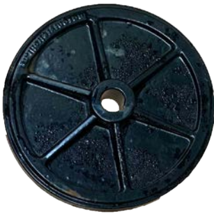
PYTHON® Starfish plate following 1500 hours of salt spray testing
