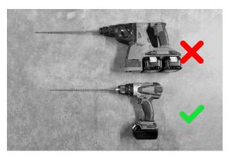
A low impact hammer drill (non-SDS) or rotary only drill must be used for drilling into all masonry materials.
