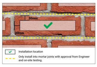
Mark the location for screw installation on the brick, at least 30mm from the brick edge.
