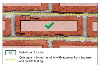
Mark the location for screw installation on the brick, at least 30mm from the brick edge.
